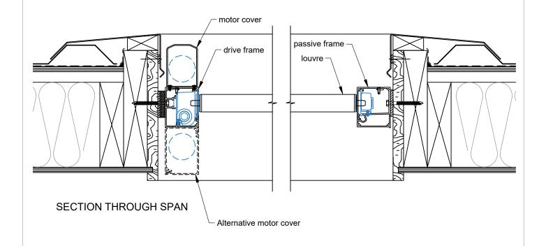
SECTION THROUGH LOUVRES - MOTORISED 200MM MAXI LOUVRE INTO EXISTING OPENING
